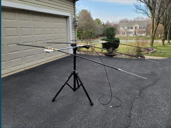
The Quick 6 meter beam was an entry from the remote site in the home brew contest by KE5NJ. The elements are attached to the boom using air chuck fittings for quick assembly and disassembly. It is claimed that after the boom is mounted to the mast the antenna can be assembled in 38 seconds.
