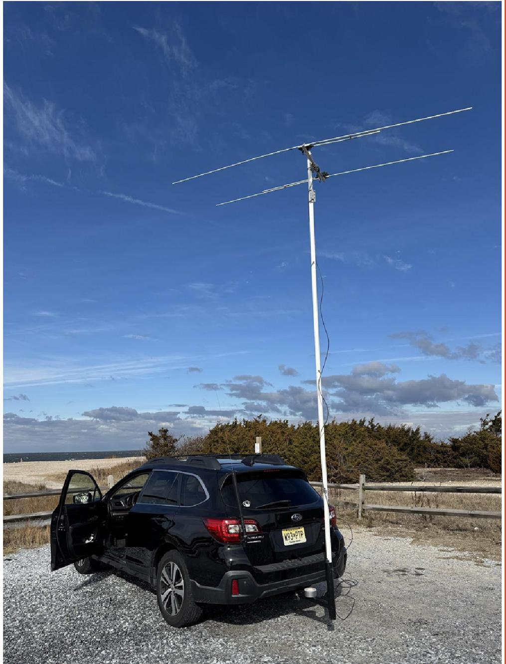
*AA2SD/R testing a 2 Element Diamond Beam with a HB9CV Configuration in Cape May NJ*
