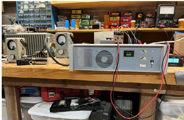
We are now working on getting a read out for the NTC thermistor so that there will be a display of pallet temperature.
