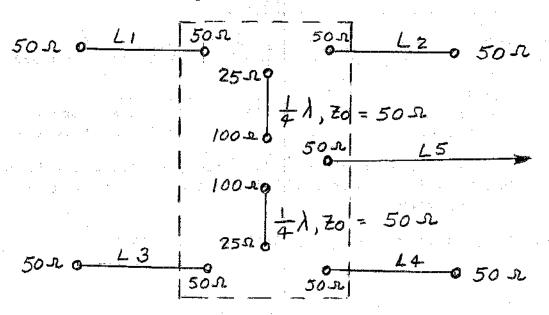
LI=LZ=L3=L4-Any length (Homemade copper hardline) L5-Any length (Feedline)
